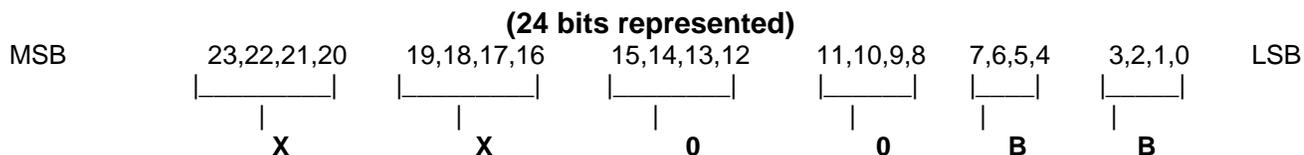
Figure 1 represents an OFFSET address of **00** Hex **XX00BB** where **XX** is the user defined MSB's, **00** is the user selectable VME-SG-GPS OFFSET and **BB** is the Board address space which is allocated for the VME-SG-GPS's I/O.
